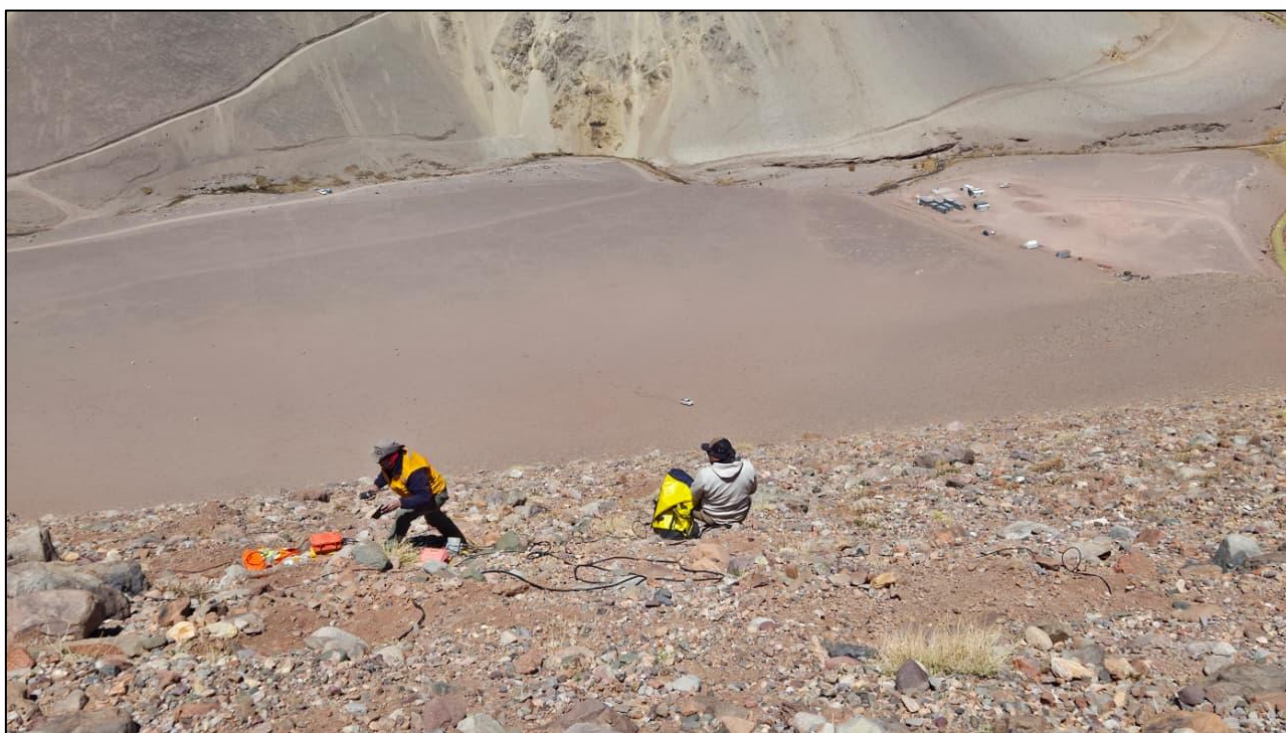
Figure 6: Quantec technicians laying out the MT/IP survey lines across the Toro targets. Note the TMT Camp in the top right corner for scale.
