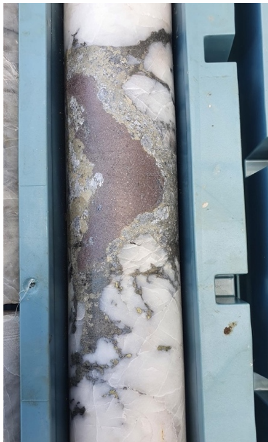
Figure 1. Hole 2: Zinc rich (pink sulphide) and copper rich (yellow sulphide) massive sulphide mineralisation at 168.13m which forms part of the 19m downhole intersection.
