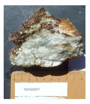
Plate A (above): TMTA00007 Toro South 'selective' rock chip sample (wet sample) with assay grades of 0.38ppm Au, 24ppm Ag & 1015ppm As.
