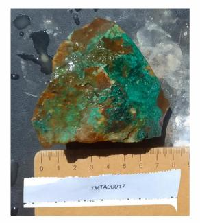
Plate A (above): TMTA00017 Toro South 'selective' rock chip sample (wet sample) with assay grades of 0.91% Cu & 0.30% Zn.
