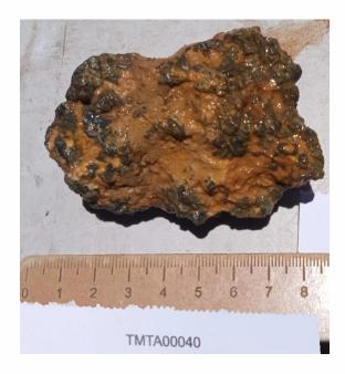
Plate B (above): TMTA00040 Toro South 'selective' rock chip sample (wet sample) with assay grades of 421ppm Ag & 20.0% Pb.
