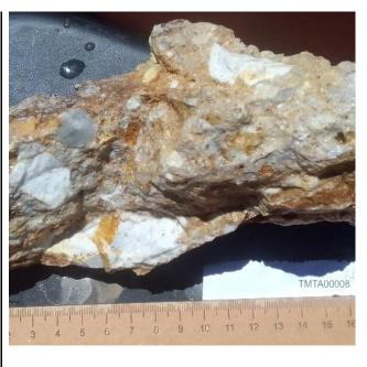
Plate C (above): TMTA00008 Toro South 'selective' rock chip sample (wet sample) with assay grades of 0.18ppm Au, 52ppm Ag, 2820ppm As.
