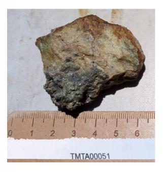
Plate C (above): TMTA00051 Toro South 'selective' rock chip sample (wet sample) with assay grades of 1.28ppm Au, 36.90ppm Ag, 0.52% Pb & 0.21% Zn.
