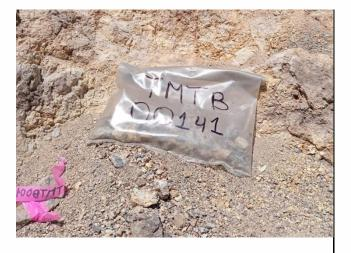
Plate A (above): TMTB00141 Toro Central 'systematic' rock chip sample (outcrop photo) with assay grades of 0.72% Cu, 6.83ppm Ag, & 1.53% Zn.
