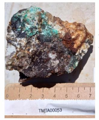
Figure 1: Toro South 'selective' rock chip sample (wet photo) with assay grades of 21.3ppm Ag & 1.41% Cu. Sample consists of a phyllic-altered dacite with sheeted manganese oxide and Cu-oxide veins that contain chalcanthite and chrysocolla. Sample Identifier: TMTA00053 located at 432482mE, 6768818mN, WGS 1984, UTM Zone 19s)
