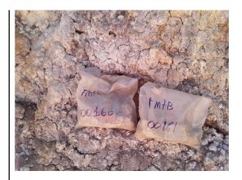
Plate C (above): TMTB00161 (Field Duplicate of TMTB00160) Toro Central 'systematic' rock chip sample (outcrop photo) with assay grades of 139ppm Ag, 0.486 ppm Au, 0.60% Zn & 0.83% Pb.
