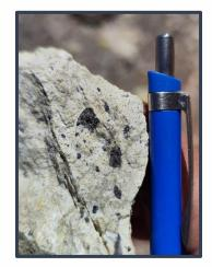
Plate B (above): TMTB00141 Toro Central 'systematic' rock chip sample (outcrop photo) with assay grades of 0.72% Cu, 6.83ppm Ag, & 1.53% Zn.
