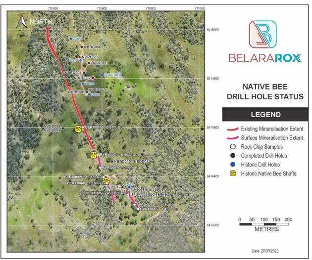
*Figure 6.* Selected rock chip samples and Phase 2 completed drill holes at Native Bee. Only Cu results (in %) are shown here. Note the surface mineralisation extents shown in pink and a secondary lode identified to the east that has not been tested by drilling yet.
