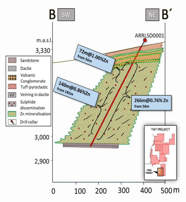
Figure 3: Due Diligence Geological Interpretation of ARRLSDD0001 along Section B-B'
