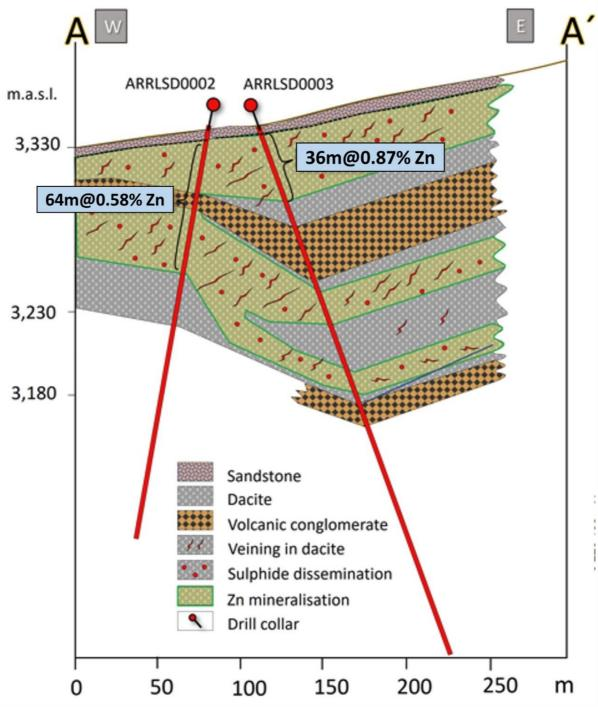
Figure 2: Due Diligence Geological Interpretation of ARRLSDD0002 & ARRLSDD0003 along Section A-A'
