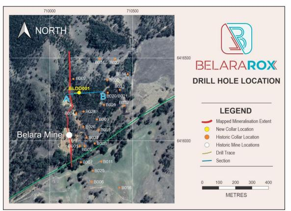
Figure 4. Drill collar location plan of drill collars at the Belara mine compared to interpreted massive sulphide mineralisation.
