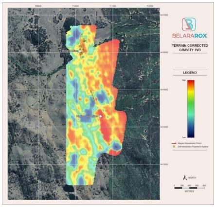
Figure 5. Gravity data with a 1VD filter applied in comparison to the extent of the known massive sulphide mineralisation and historic drill intersections projected to surface at a 0.6% Zn equivalent reported to the ASX on 24 February 2022. The chargeability high values mapped in red correspond to the known massive sulphides and extend along strike from both mines.
