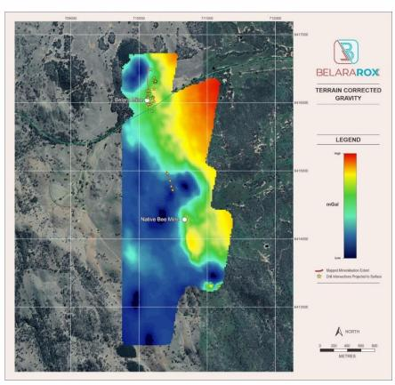
Figure 4. Terrain corrected gravity data mapped in comparison to the extent of the known massive sulphide mineralisation and historic drill intersections projected to surface at a 0.6% Zn equivalent reported to the ASX on 24 February 2022.
