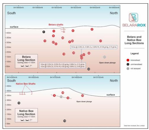
Figure 1. Long sections of drilling at Belara and the Native Bee mines (see Table 2 for intersections at a 1% zinc equivalent cut off for the relevant holes as numbered).
