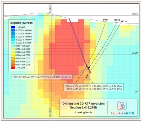
Figure 2. Cross section of drilling at Belara showing the unreported intersections in B032 and B033 compared to the mapped location of the massive sulphide mineralisation and 3D magnetic inversion model anomaly.
