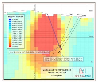
Figure 4. Cross section of drilling at Belara showing the unreported intersections in B032 and B033 compared to the mapped location of the massive sulphide mineralisation and 3D magnetic inversion model anomaly.
