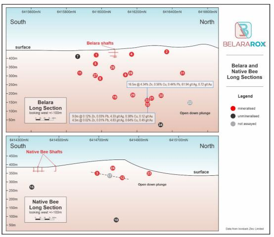
Figure 3. Long sections of drilling at Belara and the Native Bee mines (see Table 2 for intersections at a 1% zinc equivalent cut off for the relevant holes as numbered).
