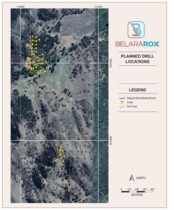
Figure 5. Drill location plan of planned resource definition holes at the Belara and Native Bee mines compared to the historic holes.
