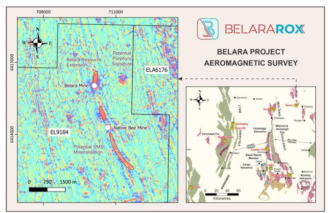
Figure1: Belara Aeromagnetic survey
