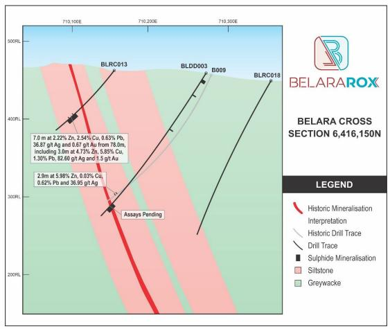
Figure 3. Section 6416150mN of drill intersection in BLRC013 relative to historic hole B009, interpreted geology and interpreted massive sulphide mineralisation from the historic model. Note BLRC018 will be completed using a diamond tail and the assays for BLD003 have not been finalised.
