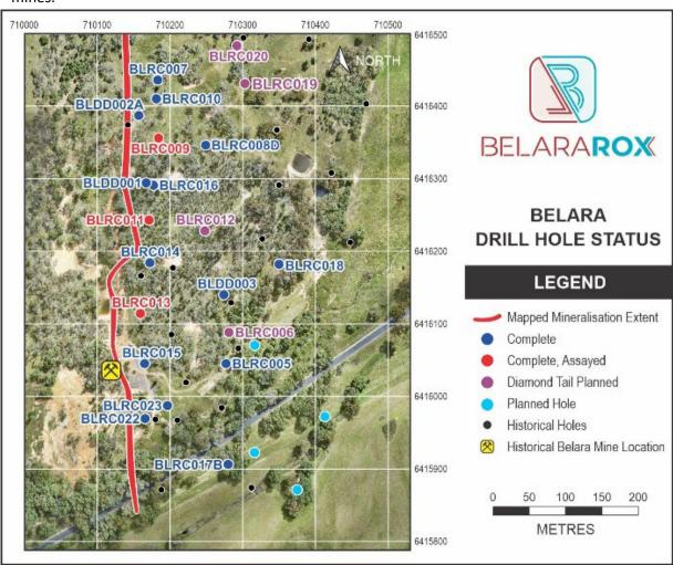
Figure 1. Drill location plan of resource definition holes at the Belara mine compared to the historic holes.
