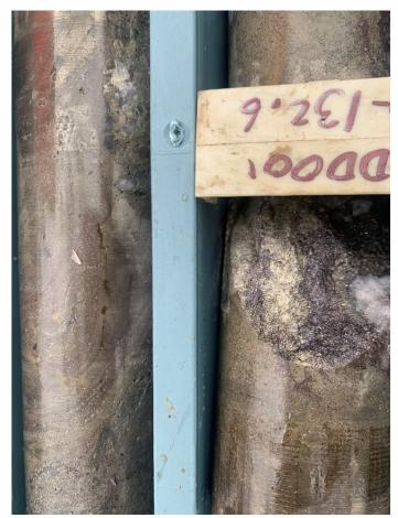
Figure 1. Zinc rich massive sulphide mineralisation at 132.6m.
