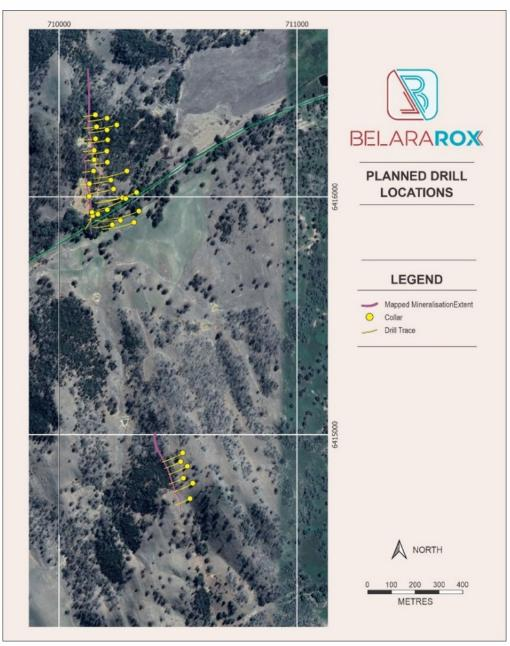
Figure 3. Drill location plan of planned resource definition holes at the Belara and Native Bee mines compared to the historic holes.
