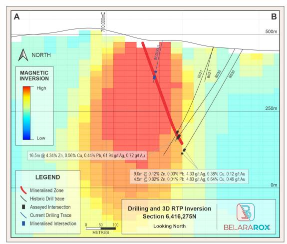
Figure 5. Visible sulphide logged in Hole BLDD001 compared to historic drilling, interpreted massive sulphide mineralisation and 3D RPT magnetic inversion.
