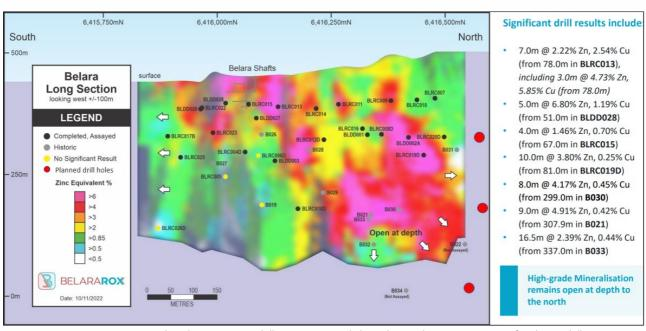
Figure 7. Long section at Belara showing existing drill intersections and planned mineralisation intersections for Phase 2 drilling
